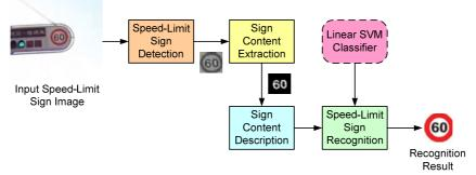
Fig. 1 Block diagram of the proposed SLS detection and recognition system.
